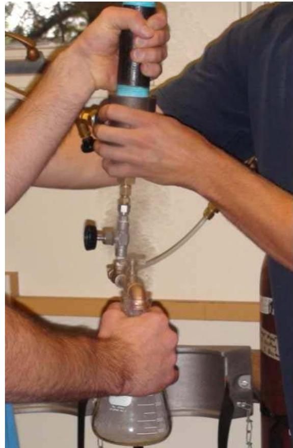
**Figure 6: Throttling procedure using rapid pressure release**
